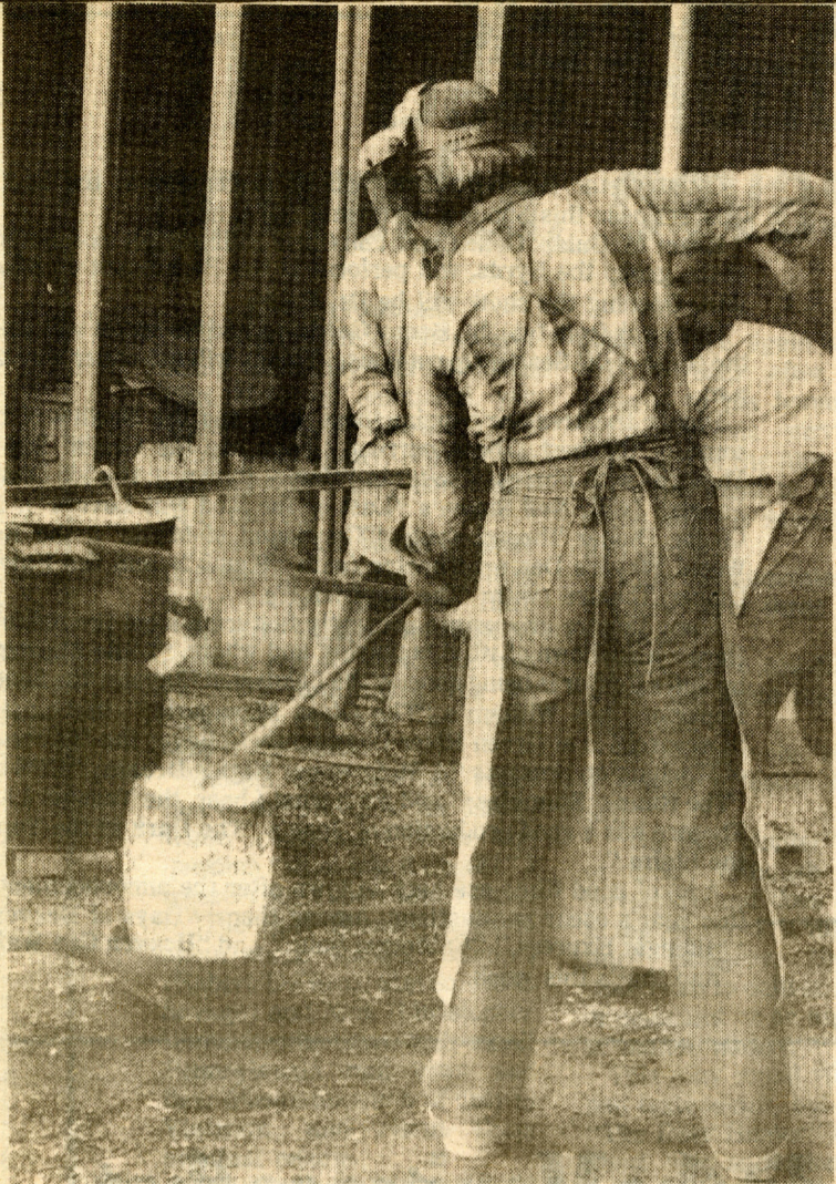
Removed from its furnace, a crucible glows red hot, filled with molten bronze.
