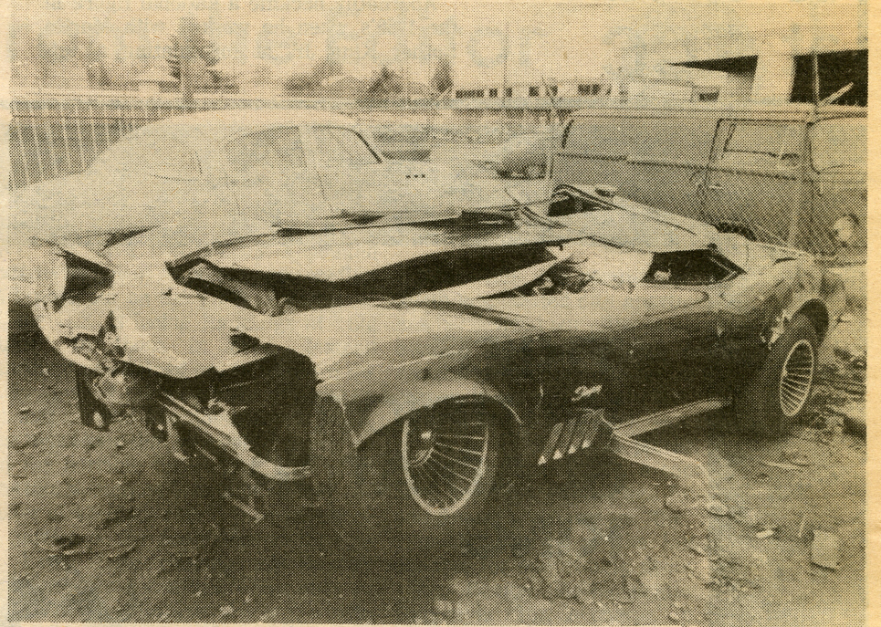
The top of the Corvette was smashed into the body when the car landed upside down.
